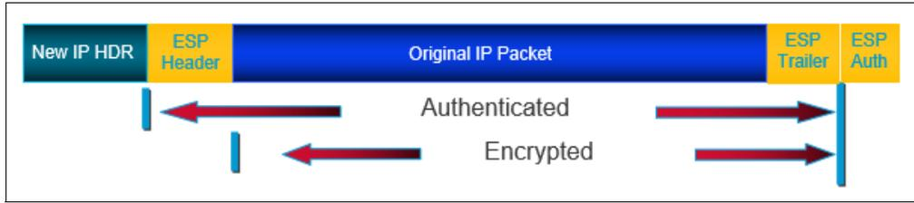
Figure 3-8 IPsec encapsulation mechanism
