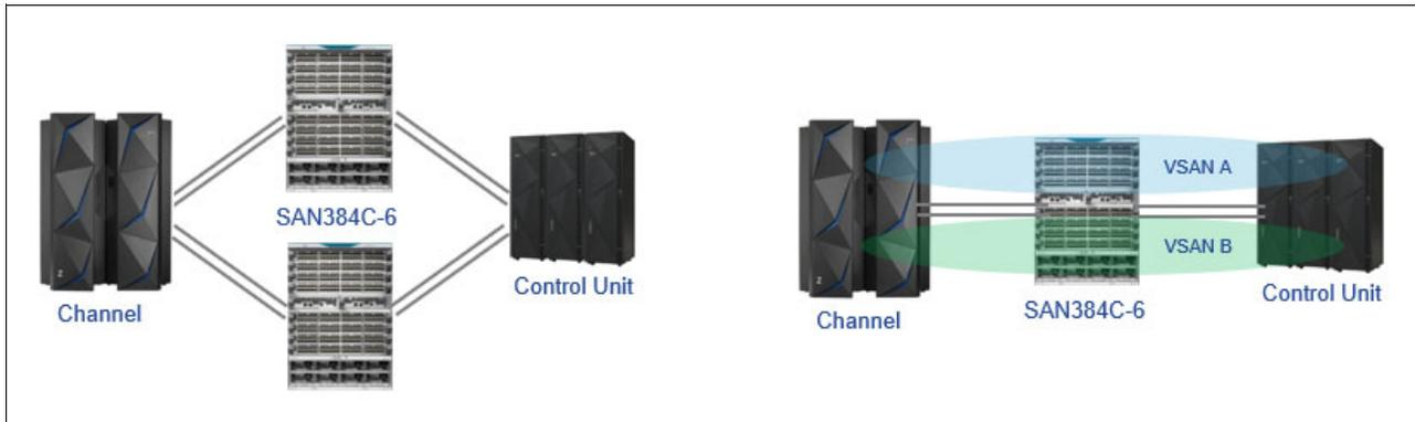
Figure 5-46 Physical versus logical redundancy
