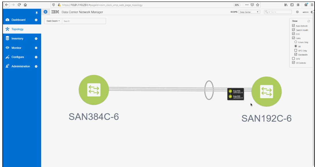
Figure 7-121 Showing the FCIP link
